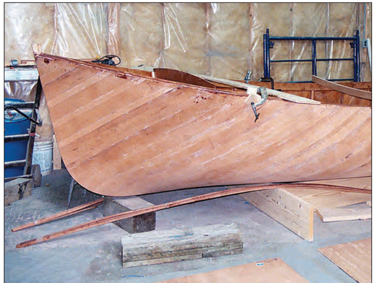
Above —Unlike its strip-built workboat predecessor, the new Six River West Pointer is cold-molded with cedar, mahogany, and epoxy. Left —Vacuum-bagging the hull as the epoxy cures results in a rigid one-piece structure that is free from voids.
