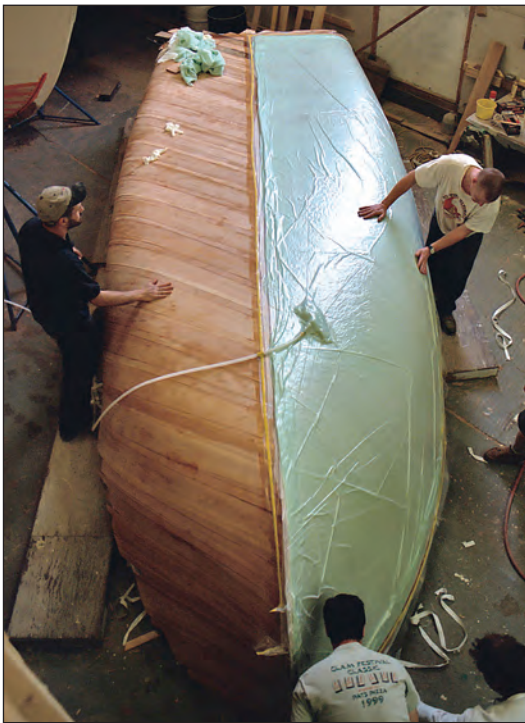
Above —Unlike its strip-built workboat predecessor, the new Six River West Pointer is cold-molded with cedar, mahogany, and epoxy. Left —Vacuum-bagging the hull as the epoxy cures results in a rigid one-piece structure that is free from voids.
